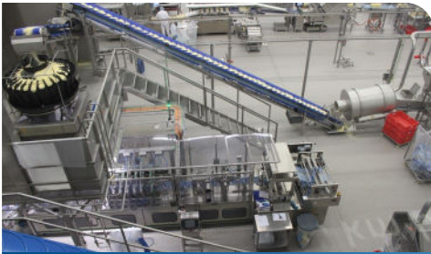
The new line produces, packs and features 100 bags of grated cheese per minute.
